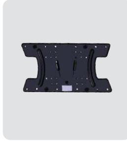
**Screen bracket** is located on the table wall. It is possible also to mount the bracket on the opposite wall. Option includes mounting plate for the wall, and mounting plate for the screen. Screen is not included. **Screen specifications:** Max. display size 50", Max. weight: 30 kg / 66 lbs **Vesa support:** 100 x 100, 100 x 150, 150 x 100, 200 x 100, 100 x 200, 200 x 200, 300 x 200, 400 x 200. As an option, compatible with Framery 2Q Lounge and Without Furniture.
