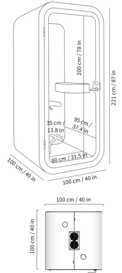
Power cord can be led out of the bottom corner of the pod.
